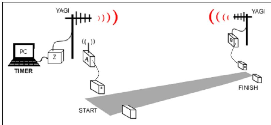
The three T-Link units are the heart of the wireless system. Each unit has a specialized purpose, and is clearly marked on the bottom with a letter to identify its function – A, B or Z. The A T-Link unit manages the start sensor, the B T-Link unit manages the finish sensor, and the Z T-Link unit acts as a go-between for the A and B units and the Timing Computer.
